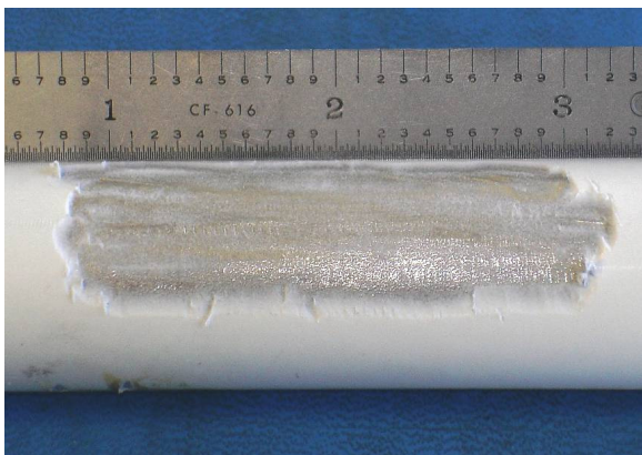
Coating scraped from frame part; damaged area approximately 2 inches (5 cm) long
