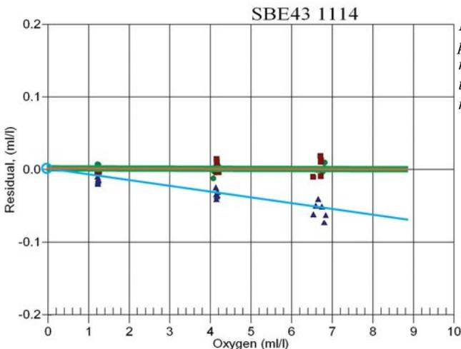
**Figure 2.** SBE 43 sensor SN 1114 original factory calibration (green dots); post-recovery calibration prior to sensor cleaning (blue triangles); re-calibration after sensor cleaning (red squares). Note the loss of sensitivity in the post-recovery calibration (blue triangles) is strictly linear, and that cleaning restored the SBE 43 to its pre-deployment calibration accuracy (red squares).
