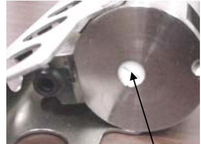
Standard pressure sensor port plug. (Note: Photo is SBE 37-SM. Pressure port details are similar for all instruments included in this application note)
