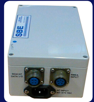
Example: PN 90488.2 SeaCAT/Sealogger RS-232 & Navigation Interface Box
