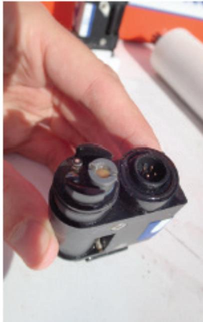
The pictures to the left show the outside of an instrument deployed at Shilshole Bay as well as what the pH sensor looks like when removed from the internal flow path. The internal pump and flow path used in the HydroCAT-EP help protect the pH sensor from accumulating biological growth, therefore limiting drift due to biofouling.
