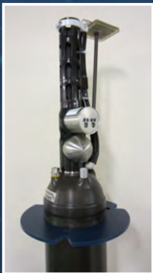
Profiling float head with integrated optical sensors
