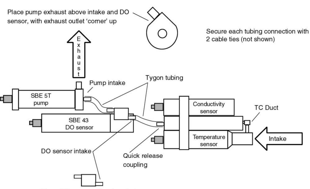
Place DO sensor with exhaust above intake, oriented as shown (± 45°)
