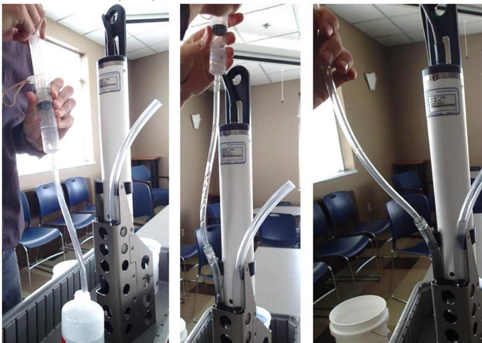
6. Flush the flow path: push the syringe in and out to flush the plumbing and sensors for the desired amount of time. Maintain at least 3-5 cm of fluid head on both sides.
