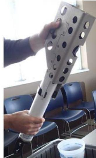
8. If a significant amount of material drains from the sensor, repeat steps 4-7 until the fluid is free of sediment.
