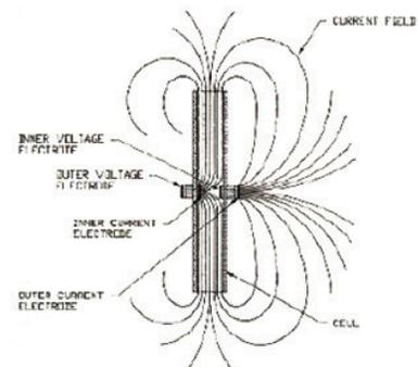
Unlike inductive and other electrode cells, the Sea-Bird Scientific cell (below) has zero external field because its outer electrodes are connected together; no voltage difference exists to create an external electrical current. The sample volume - entirely determined by the cell's hard parts - is immune to proximity errors and readily protected from fouling by anti-biology (toxic) gatekeepers placed at the ends of the cell.
