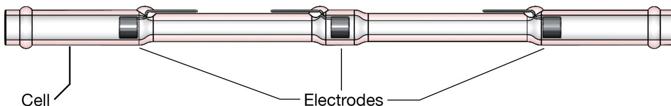
Recall that the conductivity measurement depends on the length and cross-sectional area of the volume of water through which electrical current actually flows. A fully internal field constrains the sampled volume to the cell's hard parts, and ensures that the current field flows only through the seawater sample.
