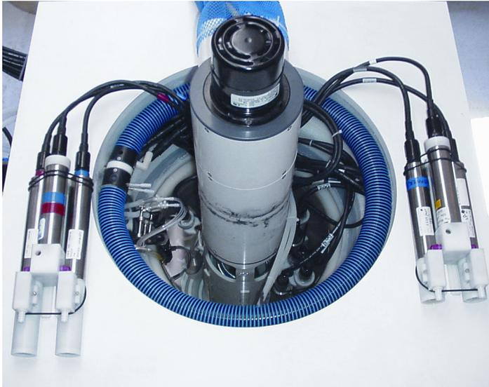
Eight SBE 43 sensors (in pumped pairs) are calibrated at one time in a computer-controlled bath.
