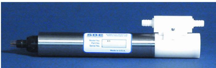
*The entire sensor with high pressure housing for electronics and plenum attached. Water to be measured is pumped through the plenum past the sensor head. If needed, poison cylinders (not shown) can be added to the inlet and exhaust ports of the plenum.*
