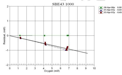
Fig. 4 Calibration results of oxygen concentration (x-axis) and the residual concentrations (y-axis) between replicate Winkler water samples and SBE 43 sensor values in a temperature controlled calibration bath. Dots specify the original calibration; triangles show post-calibration results (prior to cleaning) and the squares denote the final calibration results (after cleaning).
