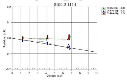
Fig. 2 Calibration results of oxygen concentration (x-axis) and residual concentrations (y-axis) between replicate Winkler water samples and SBE 43 sensor values in a temperature-controlled bath. Dots specify the original calibration, triangles show post-calibration results (prior to cleaning), and squares denote the final calibration results (after cleaning).
