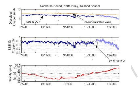
Fig. 1 Near-bed oxygen and salinity at the North buoy in Cockburn Sound for period June 26 – December 22, 2006. SBE 43 sensor 0986 was recovered on November 9, 2006, cleaned and redeployed on a different mooring and is still in the field. Top Panel: Time series of sea-bed measured dissolved oxygen (blue Jun-Nov; purple Nov-Dec) and theoretical saturation concentration (gold); Middle Panel: ratio of SBE 43 measured oxygen to oxygen saturation; Bottom Panel: sea-bed salinity.
