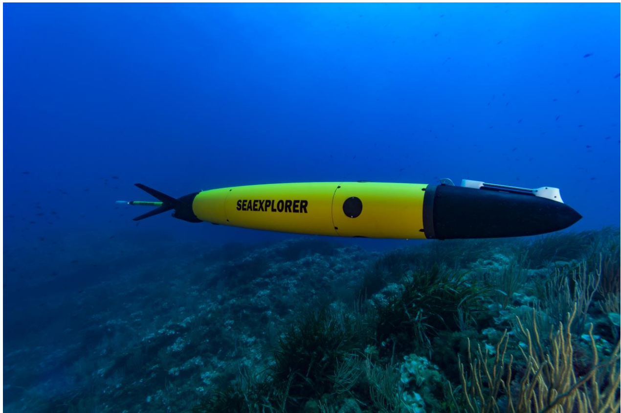
Fig 2. Side profile of the SeaExplorer glider, with the GPCTD's T-C intake sail visible in the front. When installed in the glider, the T-C intake sail sits outside of the glider's boundary layer to minimize sampling error and connect the conductivity, temperature, and optional dissolved oxygen sensors. A pressure-proof casing houses the GPCTD's electronics for installation within the glider's flooded volume.
