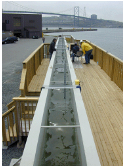
Fig. 2. The flume at Bedford Institute of Oceanography's Centre for Offshore Oil, Gas and Energy Research (COOGER) facility where the data for this comparison was collected.
