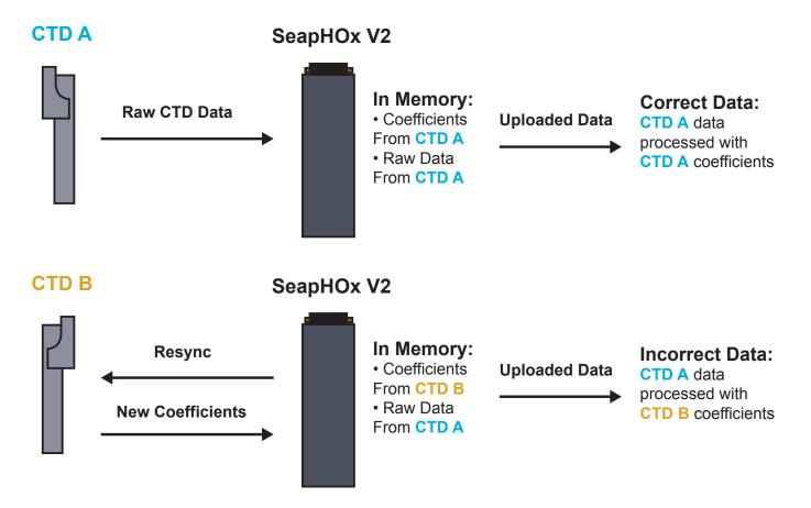
To avoid processing CTD and pH data with the incorrect calibration coefficients, **upload all SeapHOx V2 data before switching the CTD**. If this is not an option, identify the sample range encompassed by each CTD prior to switching CTDs. When uploading data, reconnect and resync each CTD and upload the appropriate samples.
