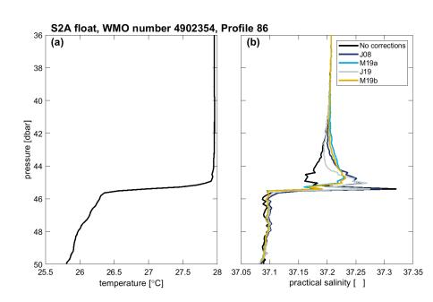
We propose a solution: add a second practical salinity data stream where dynamic corrections have been applied onboard the float before bin-averaging. This allows for direct comparisons of corrected and uncorrected data, flexibility to refine dynamic corrections in the future, and retain continuity with historical Argo data.
