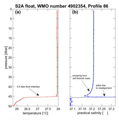
Thermal gradients (>4 °C/m) amplify dynamic errors in CTDs, salinity spiking and smearing, before corrections. Ideally, before binning CTD temperature and conductivity would be corrected for thermistor thermal mass, temperature and conductivity alignment and conductivity cell thermal mass. The data above are from a MRV SOLO-II float profiling up through the base of the mixed layer in the North Atlantic.
