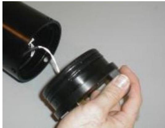
6. Remove the retaining nut.
