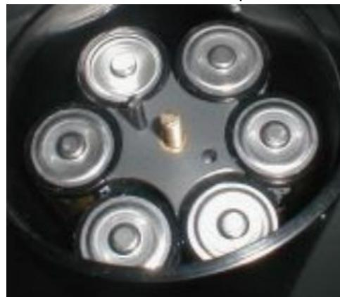
12. 51 Ah units: install four D cell batteries with the positive tab face up, in each of the other three columns marked in red.
