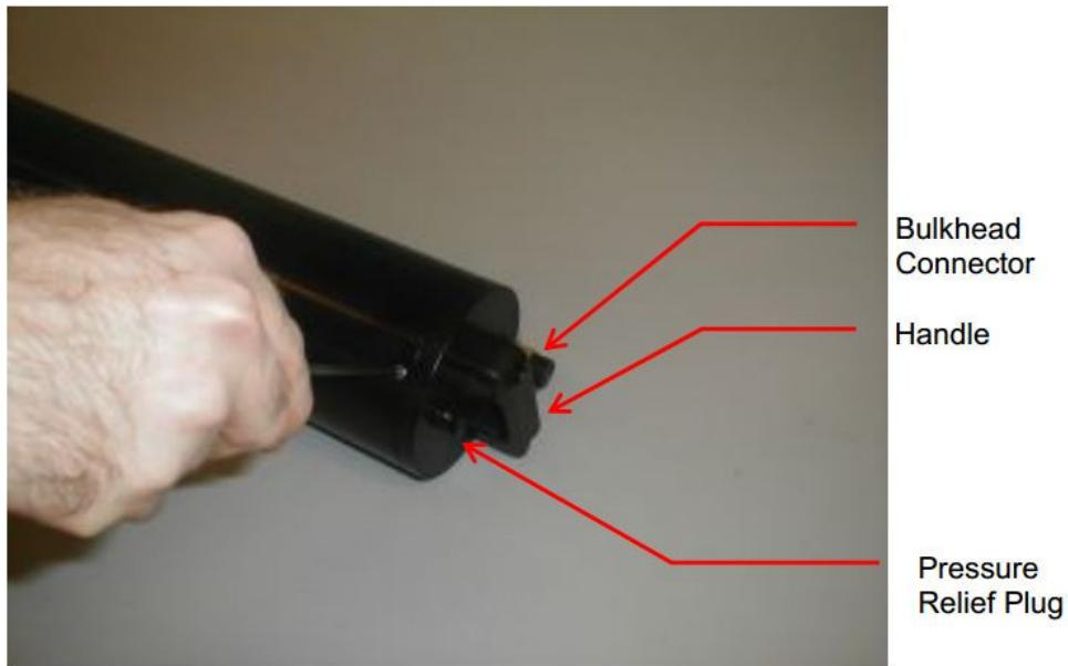
5. Disconnect the electrical connector and set the end flange aside.
