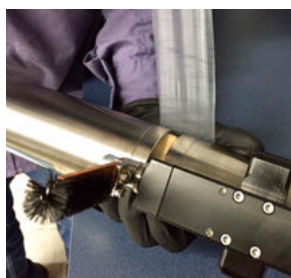
Figure 1 Parafilm® to be wound around optical area
