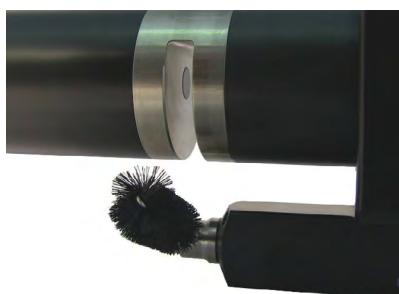
The Hydro-Wiper is an external anti-fouling system fully integrated with the SUNA V2 nitrate sensor. The Hydro-Wiper keeps the SUNA V2 sample windows clean for several months and is specifically intended for use in freshwater and coastal systems.
