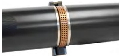
The anti-fouling guard provides passive fouling prevention through the release of copper ions that inhibit biological growth in the area. It is intended for use in blue-ocean applications with low-to-no suspended sedimentation and/or low-to-no turbidity.
