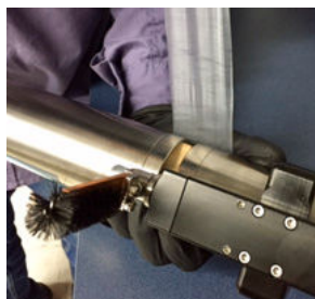
Figure 1 Parafilm® to be wound around optical area
