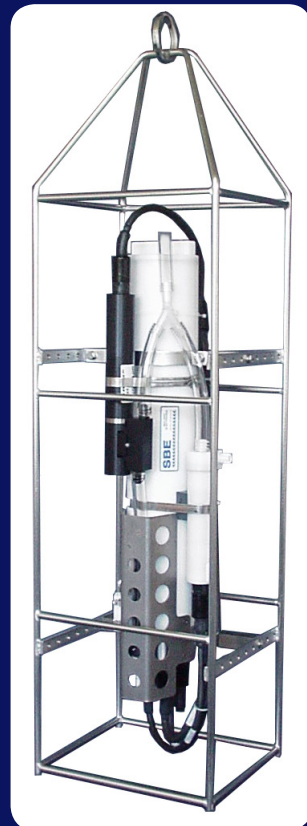
Shown with optional cage, SBE 5P pump, & SBE 43 DO sensor
