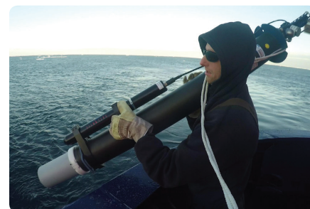
Dan Schuller of Scripps Institution of Oceanography deploys a SOCCOM float on cruise of R/V Polarstern from Cape Town, South Africa to Neumayer Station Antarctica, December 2014. Older cowlings base shown. (Photo by Hannah Zanowski, Princeton University)
